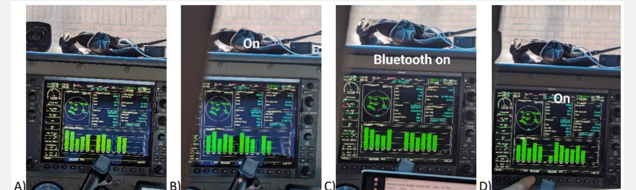
Screen captures of the Global Positioning System (GPS) signal power received from each detected satellite (one green bar per satellite) in various modes of operation of the GO-E-Stim Device: A) OFF, B) ON, C) streaming via BT, D) stimulation activated.
