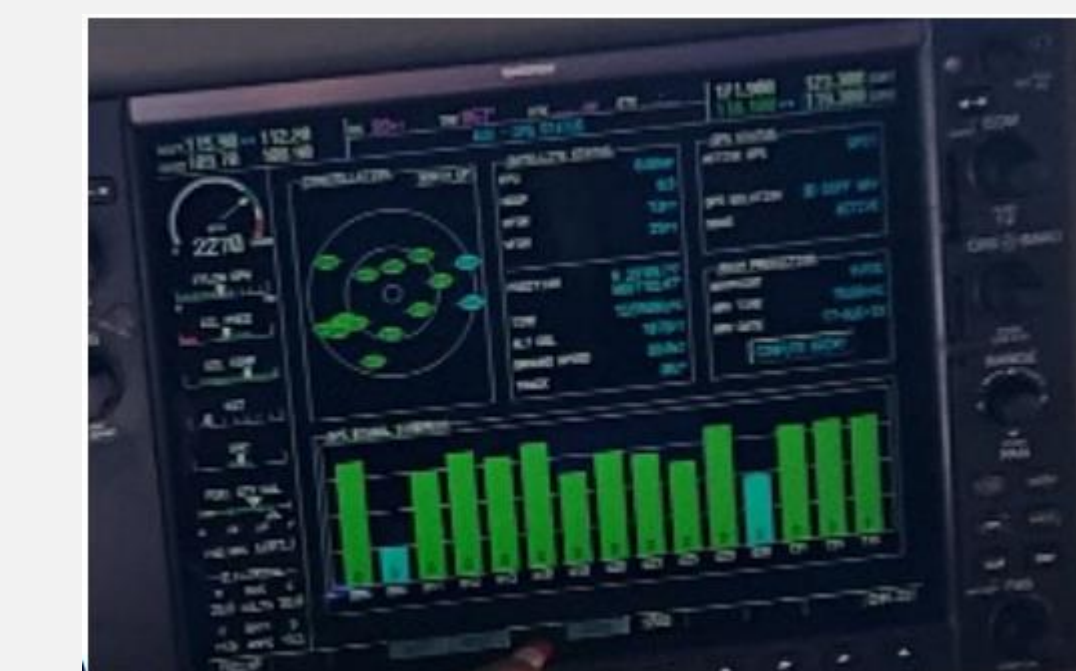
GPS signal checker detected over 13 satellites with sufficient power during flight with GO E-Stim
